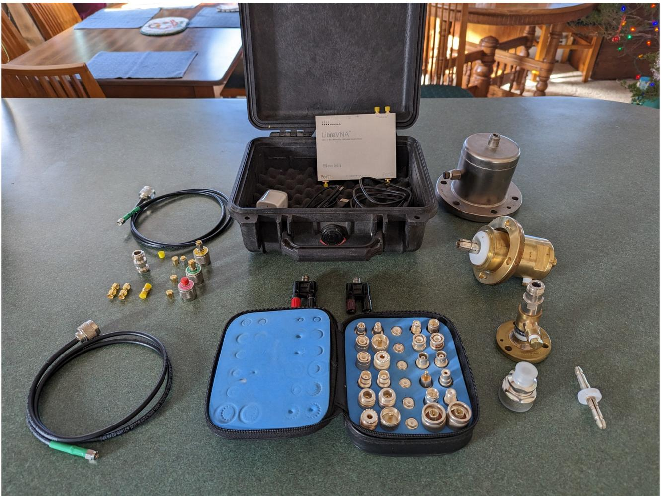
The Libra VNA is a two-port device that can make RF measurements from 100 kHz through 6 GHz with a maximum of 4501 measurement points and a maximum stimulus power of 0 dBm (0.001 watt). Higher stimulus power is important in situations where many RF signals are present that may interfere with the measurements being made. This is one case where a more expensive VNA with higher
