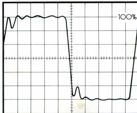
CCA Optimod-FM phase-compensated filter excited by 1kHz square wave
